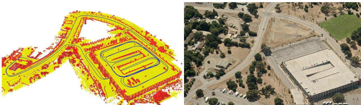
**Figure 4.21:** Corrected network from a car driving in a parking lot containing three floors multiple times (see also Figure 4.8). A multi-level surface map created from the corrected constraint network is shown in the left image. An aerial image of the same environment is shown in the right image. The images are a courtesy of Rainer Kümmerle.
