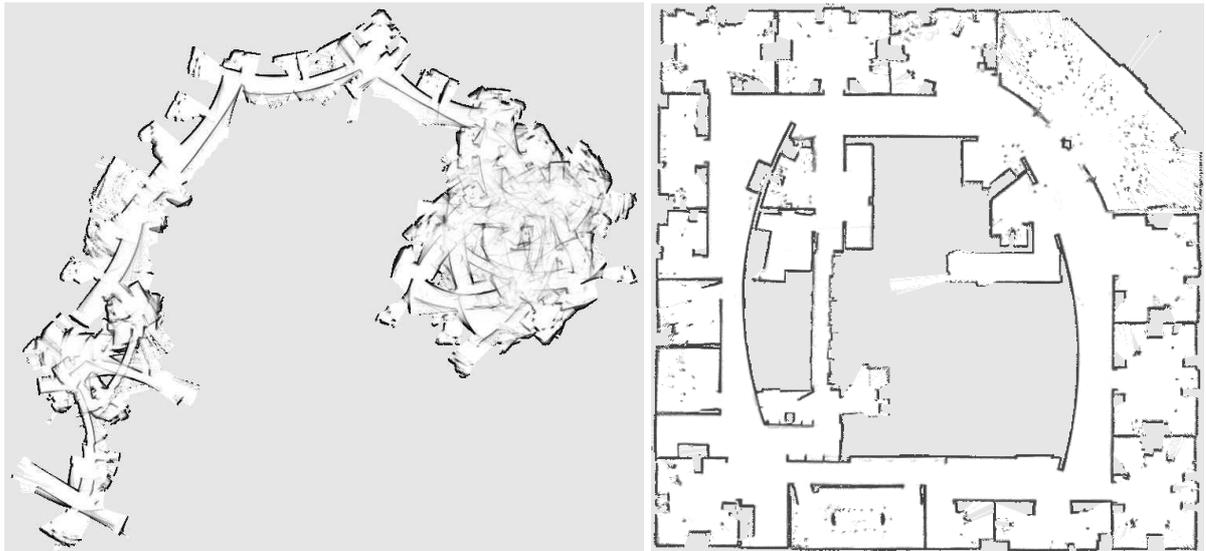
**Figure 4.13:** Two maps of the Intel Research Lab in Seattle. The left map is constructed by using the raw odometry data only. The map shown in the right image is the result obtained by using our algorithm. Here, the graph consists of approximately 1,000 nodes and about 1,800 constraints. The execution time needed to converge was less than 1 second.
